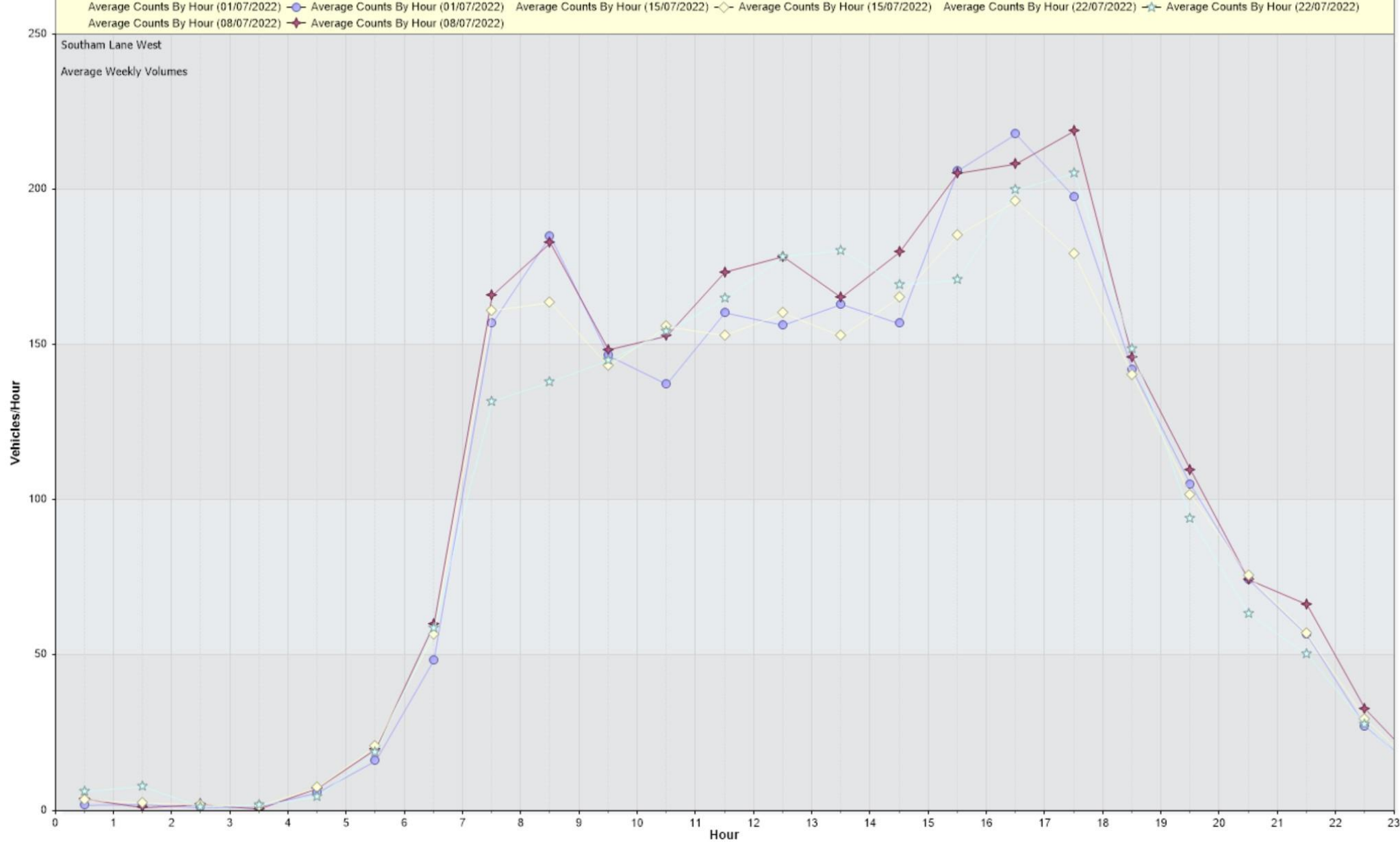
This graph shows the volume of traffic by the hour through the day, each trace represents the average over a weeks' worth of traffic volume figures.
