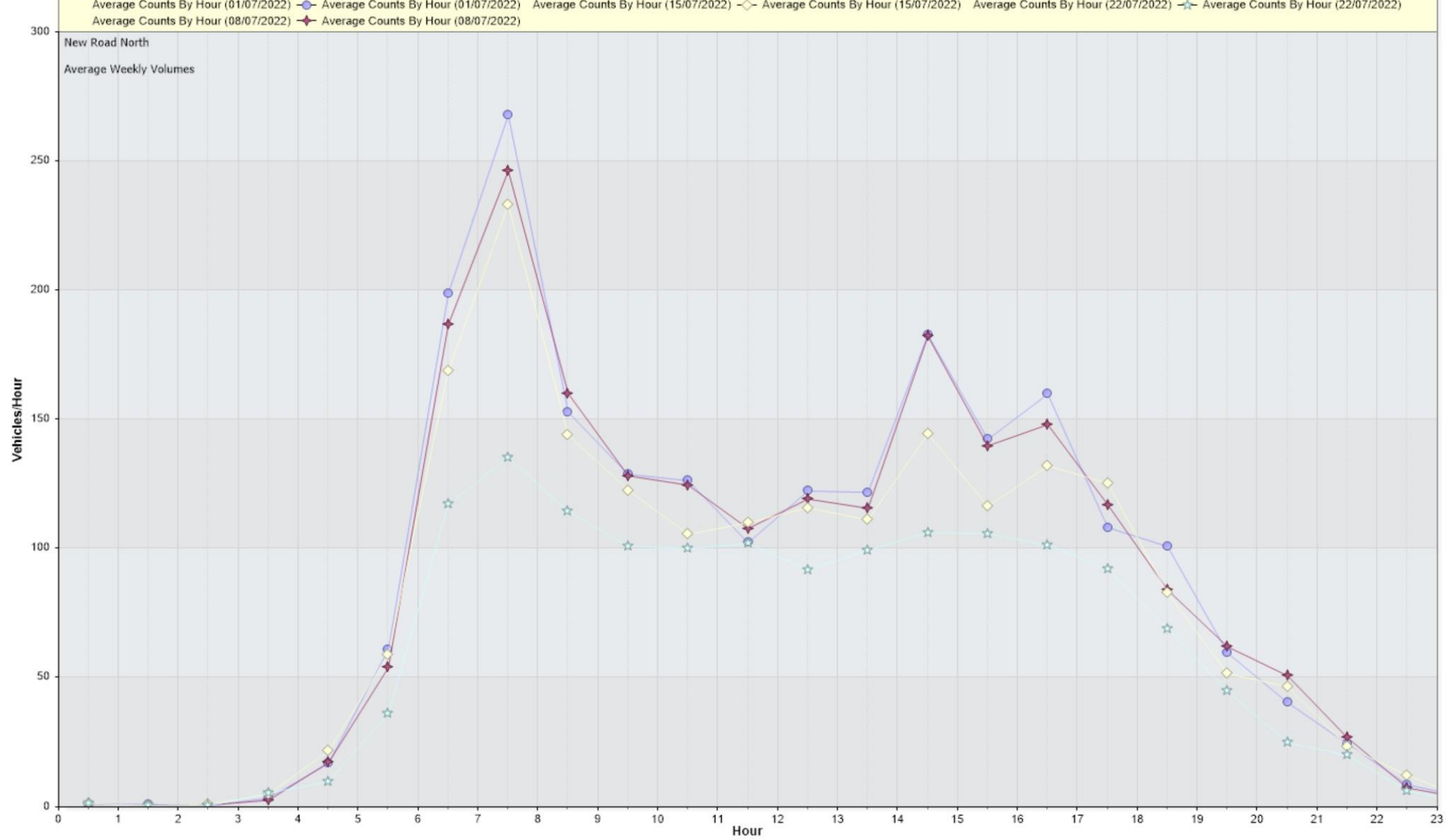
This graph shows the volume of traffic by the hour through the day, each trace represents the average over a weeks' worth of traffic volume figures
