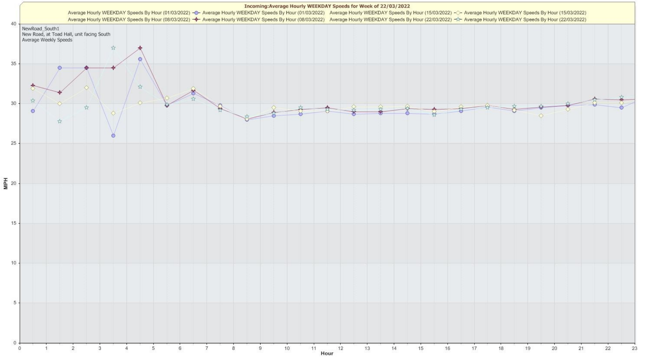
This graph shows the vehicle speeds averaged over a week, plotted by hour. It shows that the highest average vehicle speeds occur in the early morning and the late evening.
